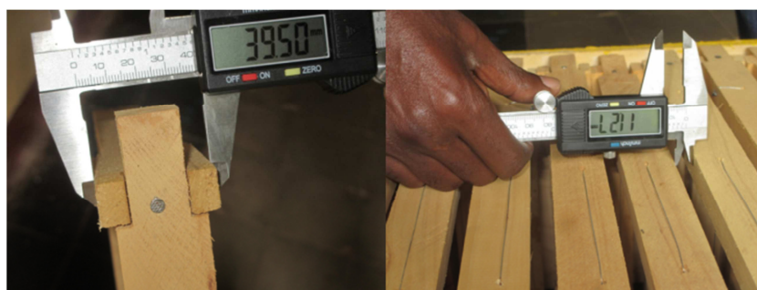
Figure 1. Measuring bar width of a frame (frame spacing, left) and bee space between two top bars of adjacent frames in movable frame box hive (right) (Photographed by author).
